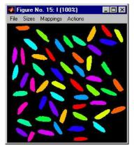
Now do the measuring. We will measure the object area in pixels ('size') and the Feret diameters ('feret'), which are the largest and smallest diameters, and the diameter perpendicular to the smallest diameter.
