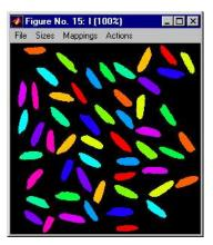
Now do the measuring. We will measure the object area in pixels ('size') and the Feret diameters ('feret'), which are the largest and smallest diameters, and the diameter perpendicular to the smallest diameter.
