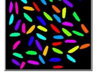
Now do the measuring. We will measure the object area in pixels ('size') and the Feret diameters ('feret'), which are the largest and smallest diameters, and the diameter perpendicular to the smallest diameter.
